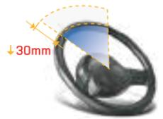
▶ The small diameter steering wheel with tilt adjustment provides the ideal operating position. The superior responsiveness of the steering wheel optimizes maneuverability even in narrow spaces.
