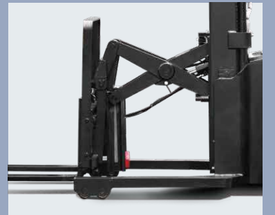
Forks move forward by the scissor structure
