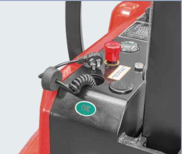
Built-in charger and maintenance free gel battery adopted to provide convenient usage
