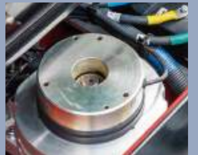
Electrical Park Brake (EPB) system
