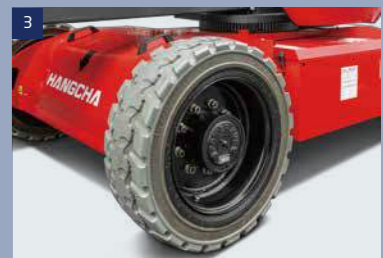
Tires: foam-filled tires with good off-road performance
