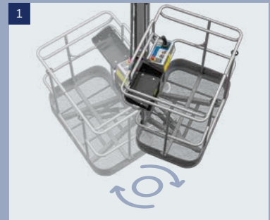
Basket: can be rotated left and right at an Angle of 140°
