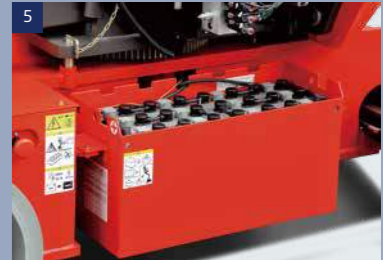
Standard tracking battery: Reduce 40% of the charge time, raise 50% of the life time
