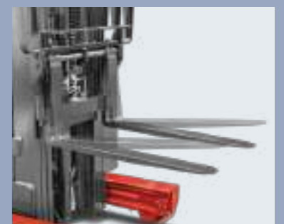
Forks can tilt forward/backward for easy loading
