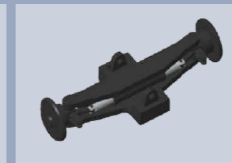
Single double-acting transverse cylinder steering axle, full hydraulic power steering and load-sensing steering gear all can provides easy steering action.
