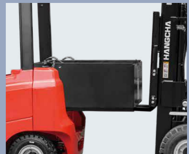
The battery can be removed from the rear enables the battery to be replaced more flexibly (Only for the lead-acid battery)
