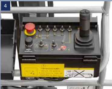
Basket control box: each action of the device can be controlled through the control box to quickly reach the working area, and the control is simple and easy to understand
