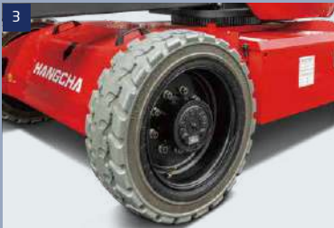
Tires: foam-filled tires with good off-road performance
