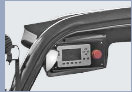
The dashboard in the driver's cab is placed overhead and can be seen when the driver lift her/his head, and the function buttons can be pressed easily
